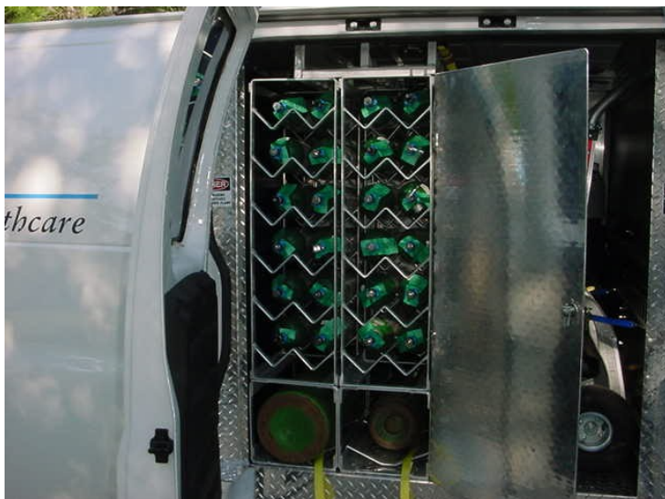
Fig 2 Typical cylinder storage rack on delivery vehicle
