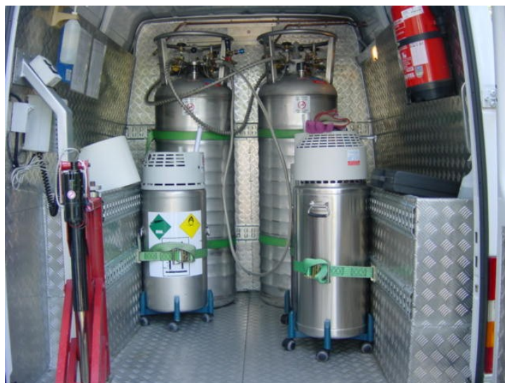
Fig 3 Typical liquid cylinder storage and security systems on delivery vehicle
