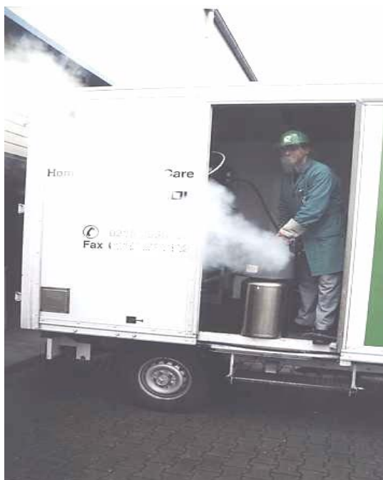
Fig 8 Typical filling of a base unit inside the vehicle with the doors open
