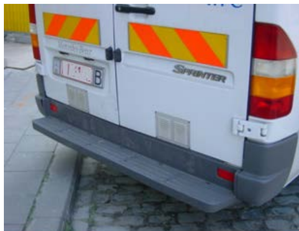
Fig 1 Typical ventilation grill at the bottom of the rear door on delivery vehicle
