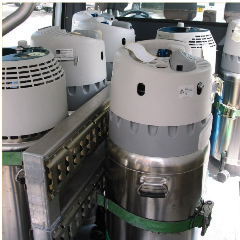
Fig 4 Typical segregation of liquid cylinders with full and empty cylinders secured separately
