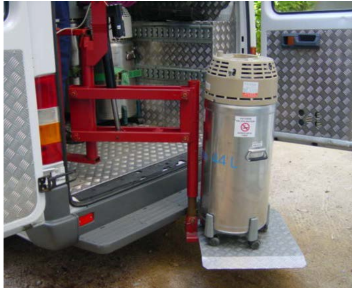
Fig 7 Typical lift used for loading full and empty cylinders in and out of the vehicle
